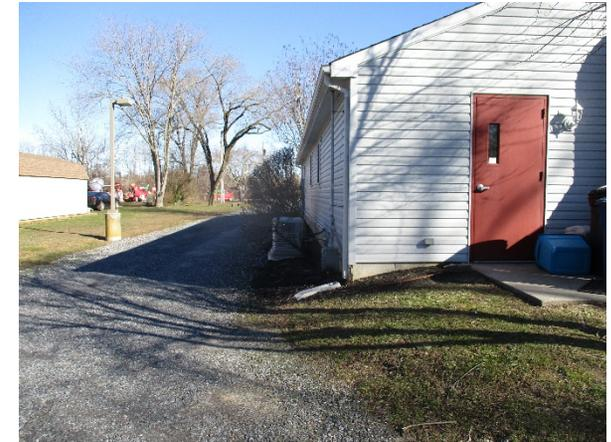
A rain garden can be installed on the southwestern side of the building to capture and infiltrate stormwater runoff from the roof of the building. Additionally, pervious pavement can be installed in the front parking lot to capture the stormwater runoff from the parking lot. A preliminary soil assessment suggests that the soils have suitable drainage characteristics for green infrastructure.
