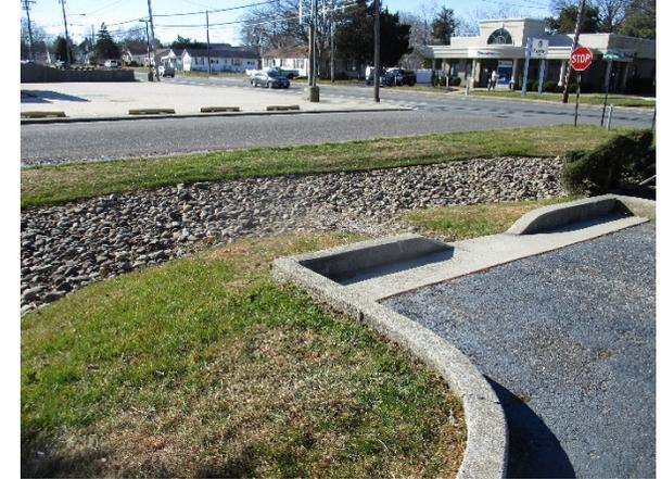
A bioretention system can be installed in the existing rock swale to capture and promote infiltration of stormwater runoff from the parking lot. Planter boxes can be installed adjacent to the building to capture and treat stormwater from the rooftop. A preliminary soil assessment suggests that the soils have suitable drainage characteristics for green infrastructure.
